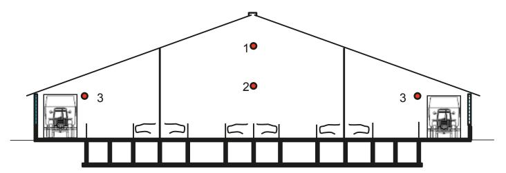
Ingoing air:  $\geq$  1 sampling point outside the house at all open side walls ( $\geq$  5 m distance). Other sources: to be considered/measured.
