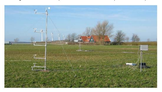
**Figure 2.** Meteorological mast holding cup anemometers to measure wind speed at five heights. In the background the centrally located mast holding the ammonia traps
