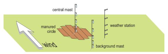
**Figure 1.** Layout of a circular plot for the measurement of NH<sub>3</sub> volatilization using the micrometeorological mass balance method, with masts supporting NH<sub>3</sub> traps at various heights in the centre of the plot and at the windward boundary of the plot.
